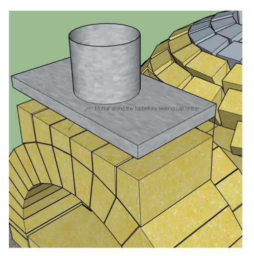
Use the airset mortar to hold the flue in place
