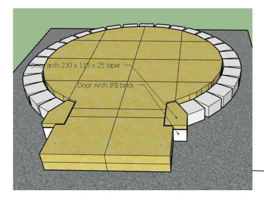
Your first layer of firebrick on the floor for your chamber consists of a White IFB. This is a strong brick that prevents any heat transfer to the slab. It also is waterproof and will never fail over time in any condition. Calcium silicate boards as a structural layer collapse over time.
