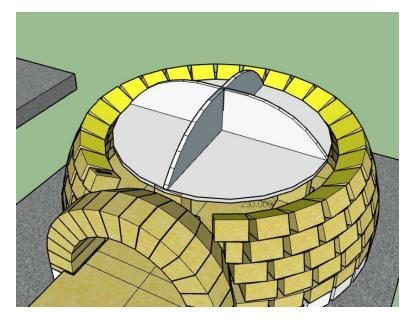
The top chamber templates simply interlock and are to be placed upon the 8 bricks with the centre line running from front to back.
