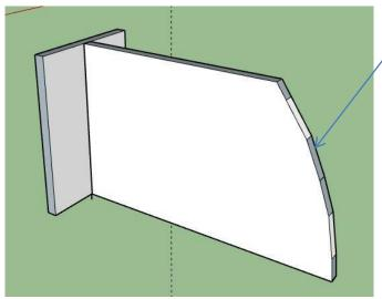
Your chamber template needs to be assembled. It consists of 2 pieces and has notches for each brick layer
