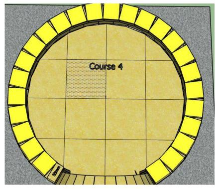
By now it's a good time to infill the rear of the chamber bricks with fondu – mix your batch and infill the rear of the chamber to strengthen it.
