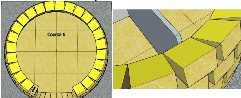
The 6<sup>th</sup> layer is your final layer before the plug to build the top of the oven. Check layer 6 meet the top of the 2<sup>nd</sup> last notch in the template
