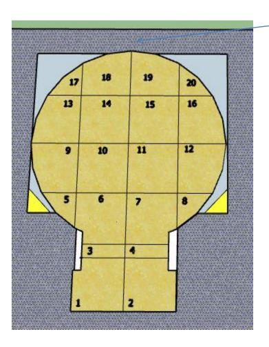
Starting from the rear edge of the calcium silicate board and in the middle join lay your tiles in the following pattern loosely
