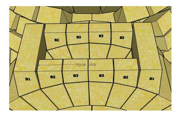
You can dry fit these first with the flue cap on top. Then Set the B1 bricks in place with the flue cap on top used the airset mortar, then using a flat edge set the b2s and b3s to get a nice finish.
