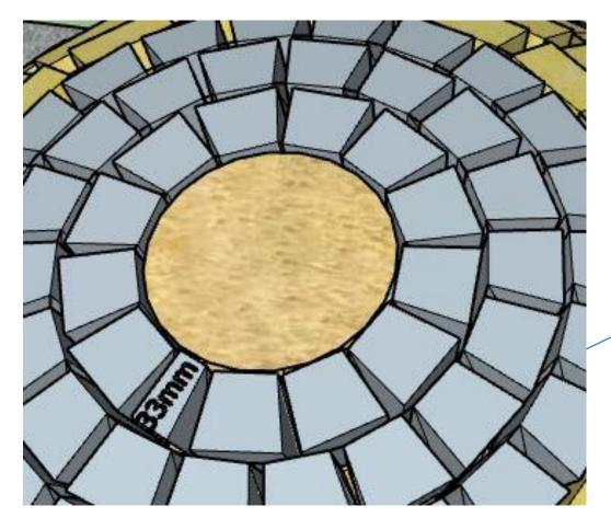
For the keystone mix some CAST 13 in a bucket and pour into the top to lock the entire structure togther.
