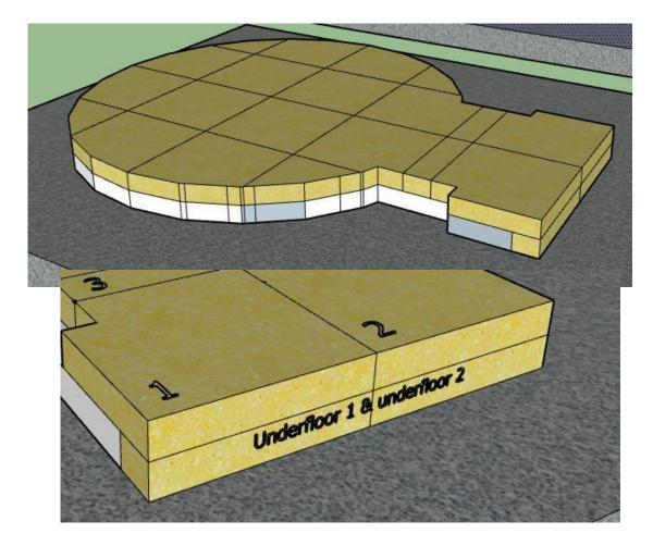
With a handsaw trim around the perimeter of the floor tiles cutting the calcium silicate board flush to the tiles ..
