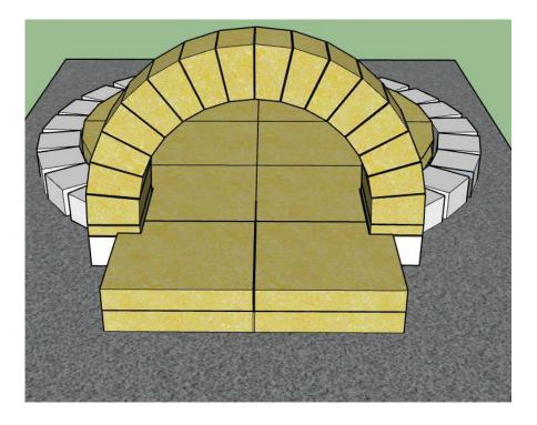
When you have finished the door arch leave the template in for at least an hour before removing it. You can also leave it in while building the chamber if you like.
