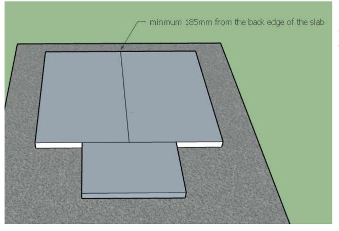
Lay your calcium silicate board in the center of the slab and 185mm from the rear of the slab
