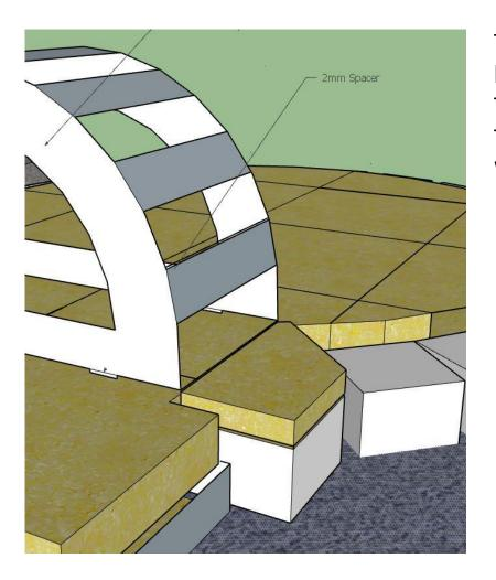
To start building your door arch only butter the bricks to 2-3 mm between bricks and Tap down gently.
