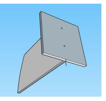
Join the template together with nails or screws from the rear in 2 places
