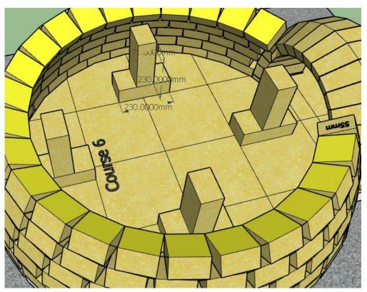
Using 8 common house bricks 230 x 115 x 75mm create 4 positions evenly spaced for the top templates to rest upon. You can put 2 more in the centre to hold it up if you like. *Placed a layer of black builders poly plastic covering the bottom of the oven and partially up the sides to catch the sand and debris when you knock out the bricks to make the clean-up easier*
