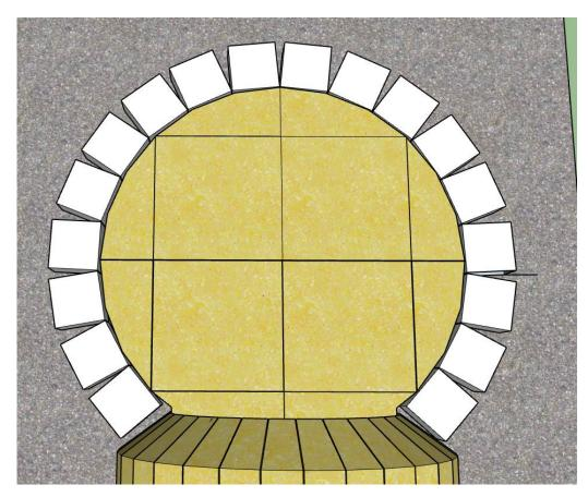
If you were supplied 50mm Calcium silicate insulation board versus the standard 25mm you will also have 115 x 115 x 25mm IFB insulation brick. These on go ontop of the first IFB layer to lift the first IFB layer levell with the cooking floor
