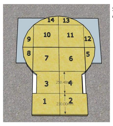
Starting from the rear edge of the calcium silicate board and in the middle join lay your tiles in the following pattern loosely
