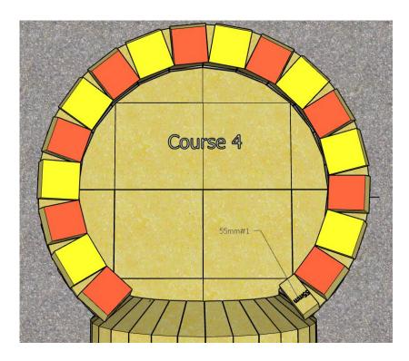
By now it's a good time to infill the rear of the chamber bricks with fondu – mix your batch and infill the rear of the chamber to strengthen it.
