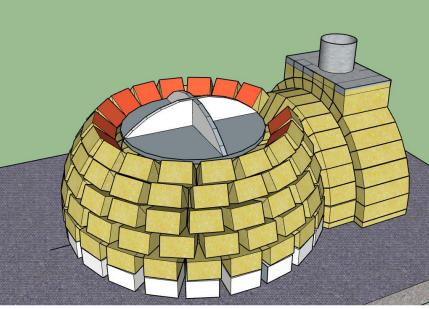
The top chamber templates simply interlock and are to be placed upon the 8 bricks with the centre line running from front to back.
