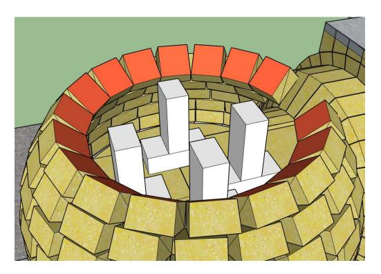
Using 8 common house bricks 230 x 115 x 75mm create 4 positions evenly spaced for the top templates to rest upon.
