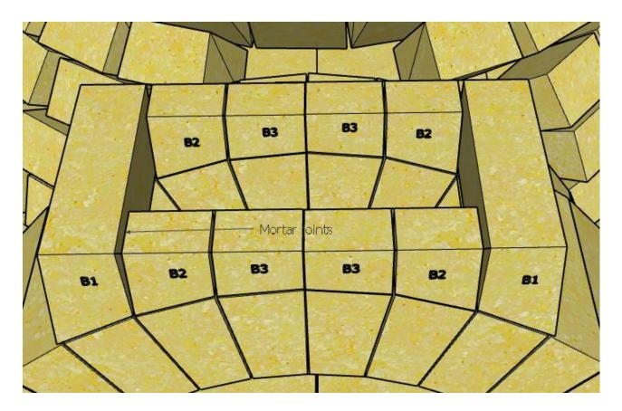
You can dry fit these first with the flue cap on top. Then Set the B1 bricks in place with the flue cap on top used the airset mortar, then using a flat edge set the b2s and b3s to get a nice finish.
