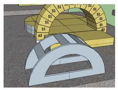
Screw or nail your door arch template ( smaller ) together using timber at approximately 180mm long - only 6 battens needed.
