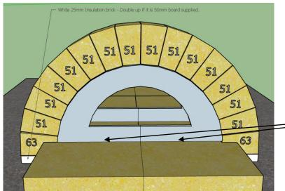
make sure you have placed 4x 2mm or (20c pieces) spacers under the door arch template so it can be removed to make the template drop instead of pulling it out in which may disrupt the bricks.
