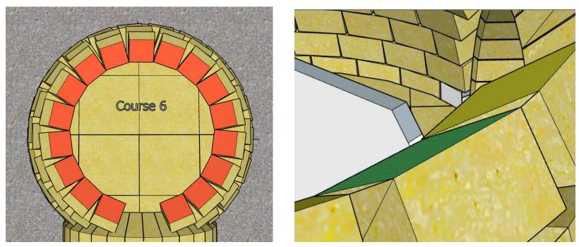
The 6<sup>th</sup> layer is your final layer before the plug to build the top of the oven. Check layer 6 meet the top of the 2<sup>nd</sup> last notch in the template
